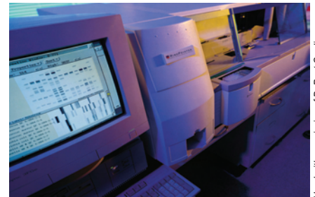
The automatic RiboPrinter® system from DuPont Qualicon identifies and characterizes bacteria through genetic "fingerprinting."
